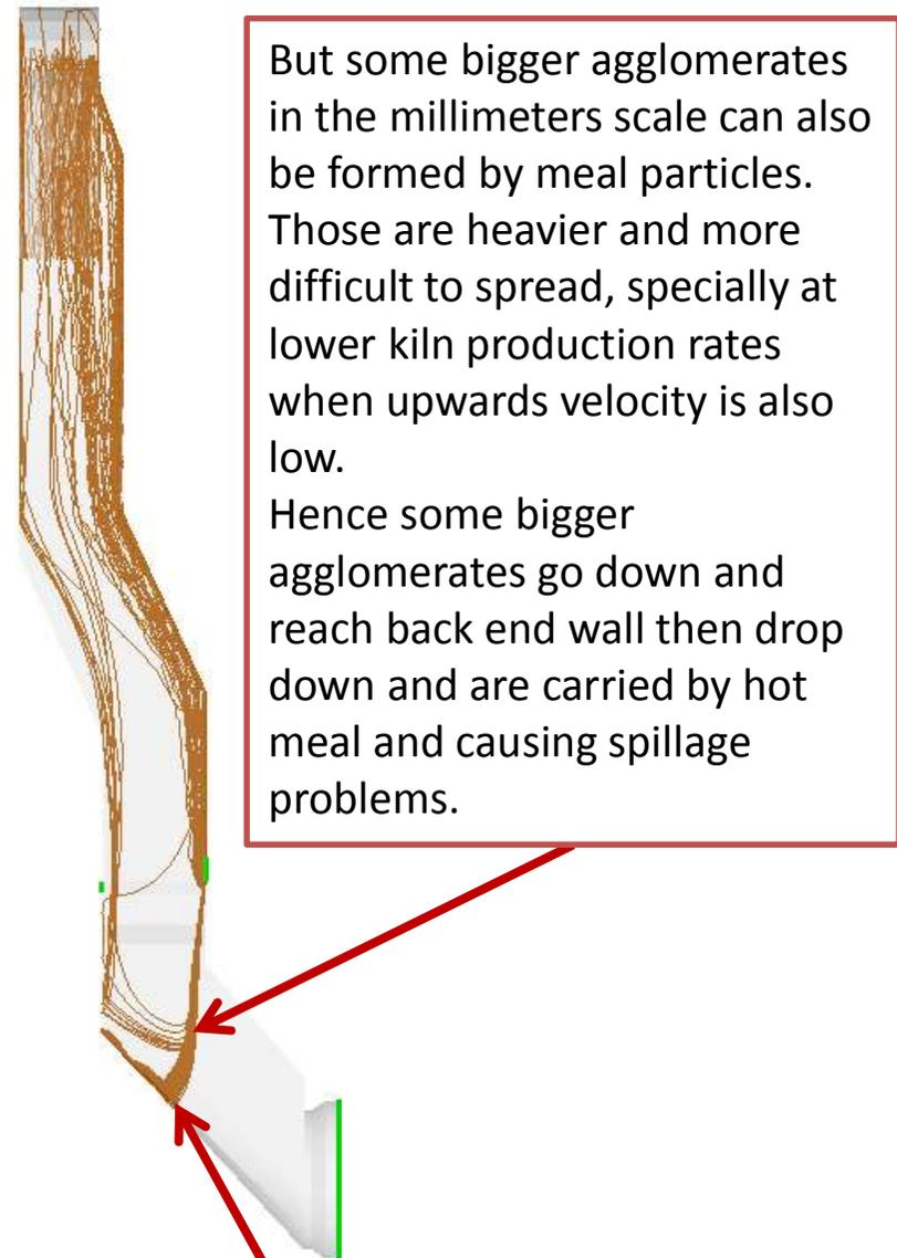
But some bigger agglomerates in the millimeters scale can also be formed by meal particles. Those are heavier and more difficult to spread, specially at lower kiln production rates when upwards velocity is also low. Hence some bigger agglomerates go down and reach back end wall then drop down and are carried by hot meal and causing spillage problems.
