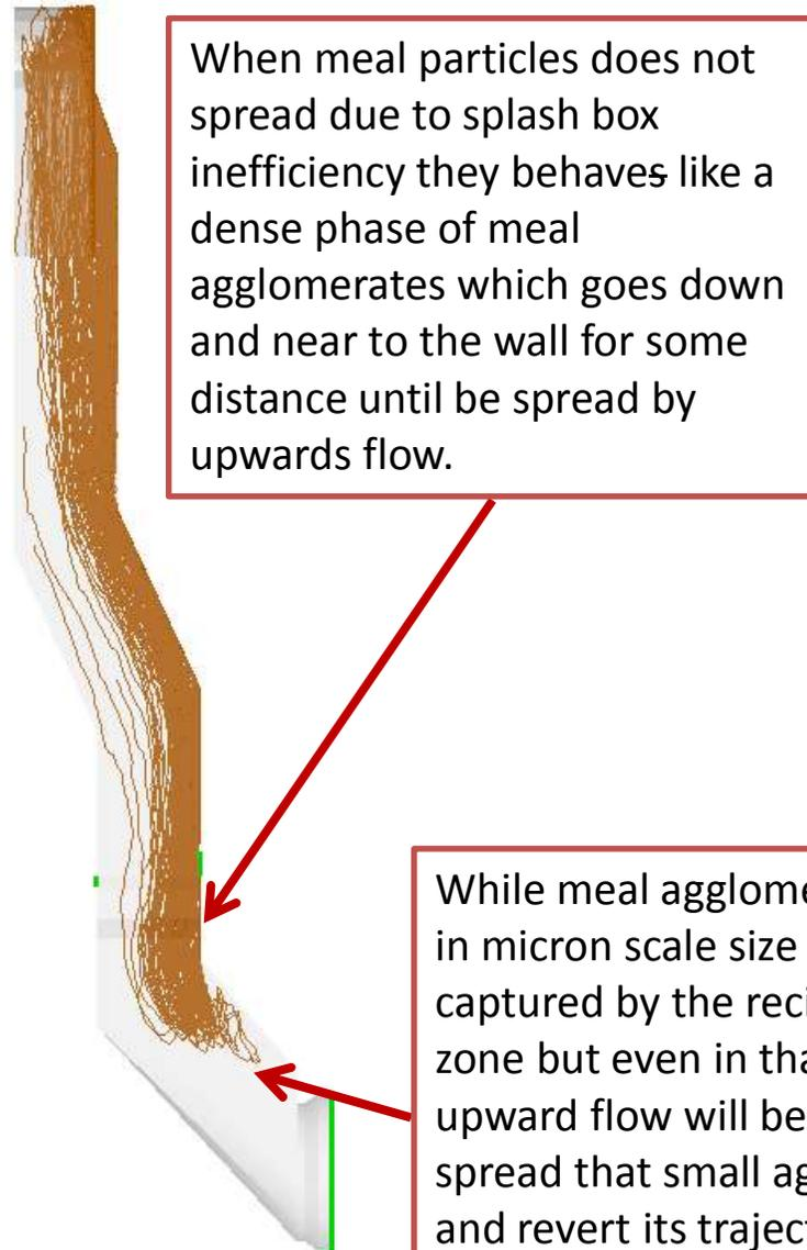
When meal particles does not spread due to splash box inefficiency they behaves like a dense phase of meal agglomerates which goes down and near to the wall for some distance until be spread by upwards flow.
